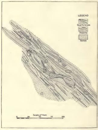
Fig. 3.—Silver Peak, Nevada. Vertical cross-section of chief stope workings, Drinkwater mine. Shows characteristic branching and lenticular form of auriferous quartz veindikes in schist. From J. E. Spurr: Professional Paper 55, U. S. Geol. Surv.; Plate XII.
